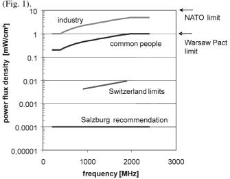
Fig.1: Limits for power flux density during RF-EMF exposure
