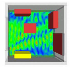
Fig 3: Interferences of electromagnetic waves (900MHz) in a room. Taken from "Forschungsbericht der IMST GmbH an das BfS"", March 2005. Reprint with kind permission of IMST GmbH
