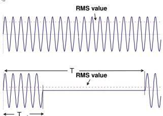
Fig 2: RMS value of a sinus form function (top) and of a pulsed sinus form function (bottom)
